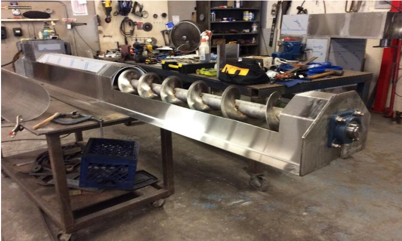
Construction Photos Depicting the Shaft and Flighting and Internal Wedge Wire Chassis that Allows for Additional Dewatering During Transport
